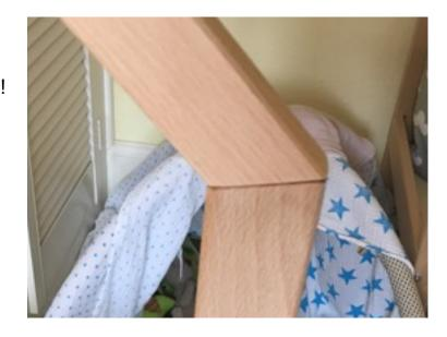
f) I need some additional timber to make the roof apex cross-bar and for a cross-bar at the back to give some extra stability. I made these from strip pine (without knots). I made the roof apex cross-bar into a L-shaped profile to give additional rigidity, and used furniture bolts with barrel nuts, plus an unglued dowel, to create each joint.
