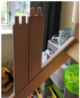
g) Lastly, I used the remaining offcuts off White Beech to make a chimney stack, which I dowelled to one of the roof-rails.
